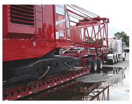
One of the most difficult pieces of equipment to transport is a crane. A Cajun Construction trailer moves a Manitowoc 4000V crane.
